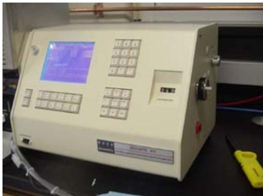
1. Press the red button on the right side panel of the machine to turn on the lamp as well as the instrument's built in computer. Wait 20 minutes before data collection for the lamp to warm up. If you need to change lamp or if the AA has not been used for a few months, align the wavelength of the lamp (see pages 16 to 17 of the manual). You may also need to align the lamp position after you change lamp.
