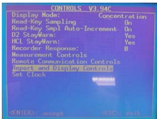
10. To adjust for the number of digits in the output, press [cntrl] and select the “Report and Display Control” menu. From there, adjust for the decimal places in the concentration or absorbance output accordingly.
